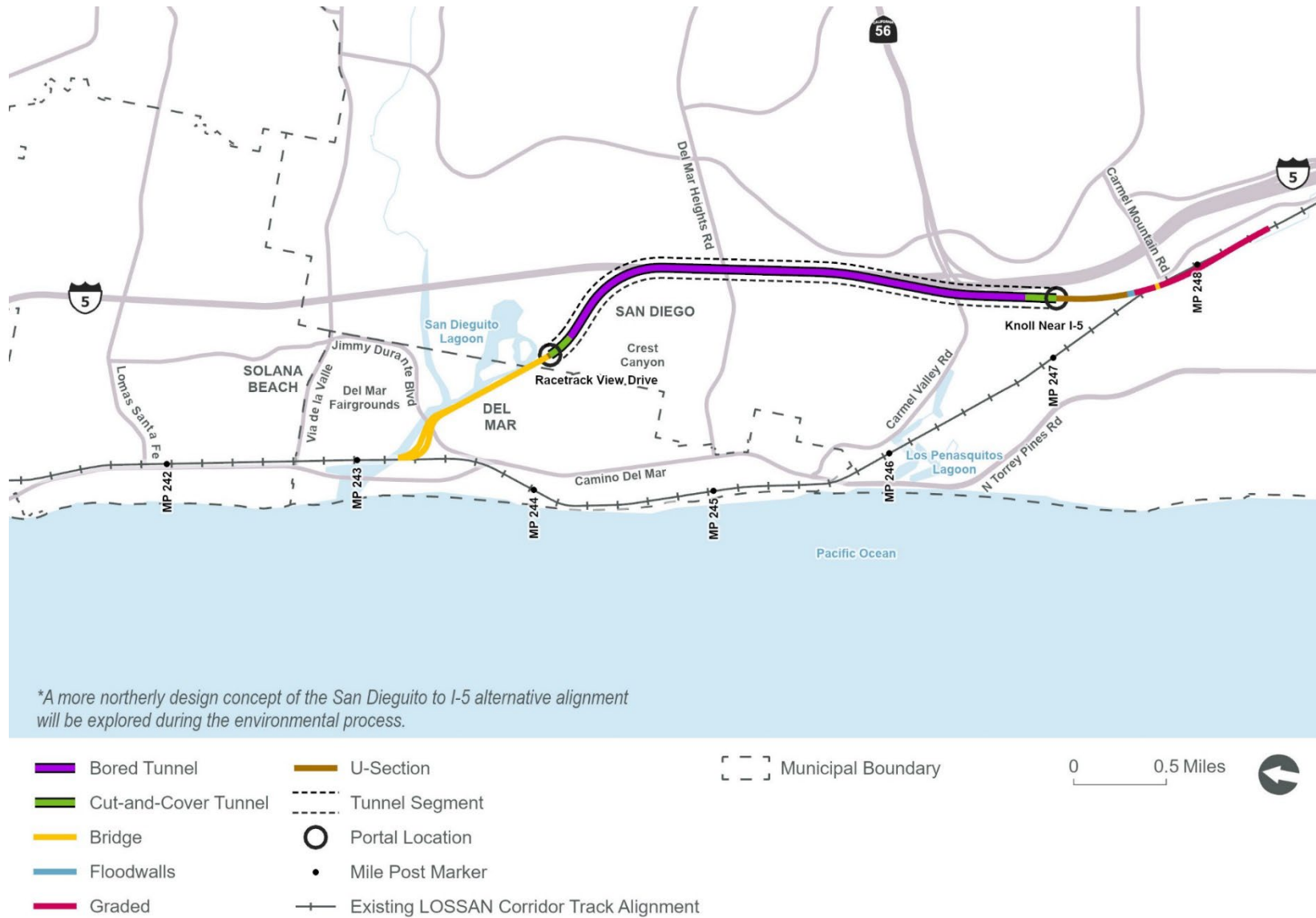
Figure 4. San Dieguito to I-5 Alternative Alignment
